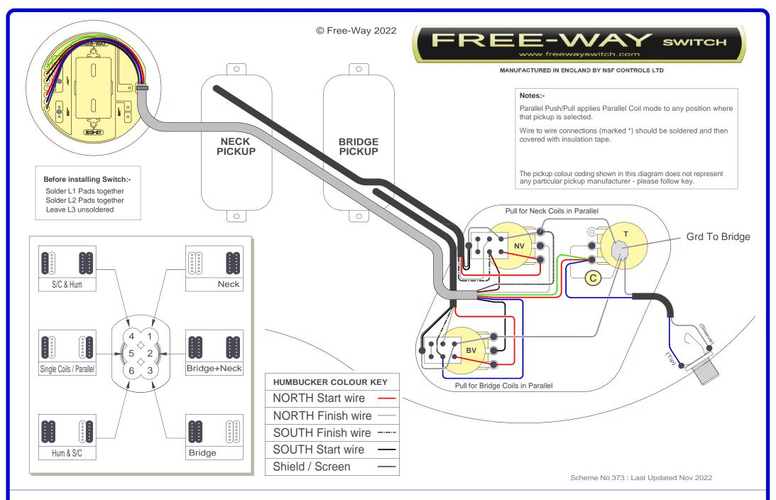
Model No:- 3X3-07 Free-Way Switch HH Hum + S/Coil Combinations + Parallel 2V1T
